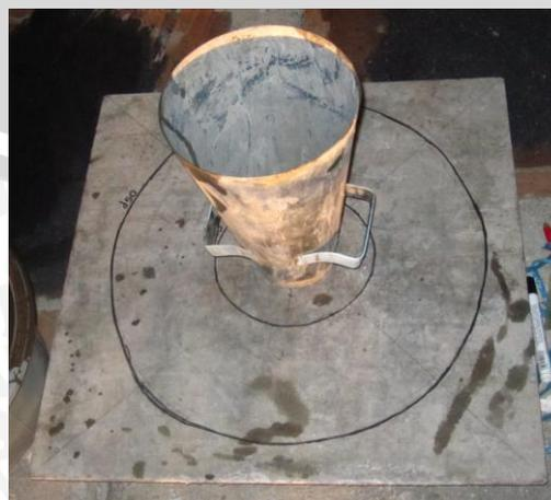
**Gambar 2.3** *Slump cone*
