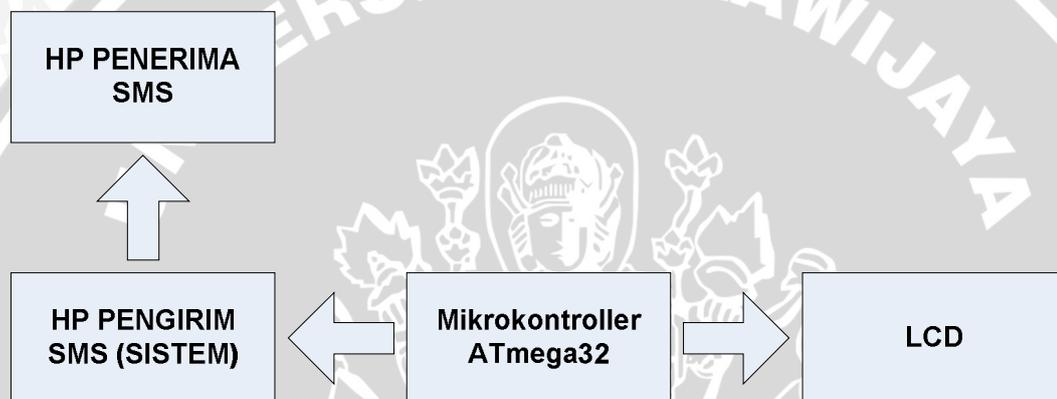
**Gambar 5.41.** Blok diagram pengujian pengiriman SMS
