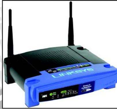
Gambar 4. 2 Access point router WRT54GL
