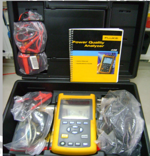
Gambar 4.3. Alat Ukur Power Quality Analyzer Fluke 41B
