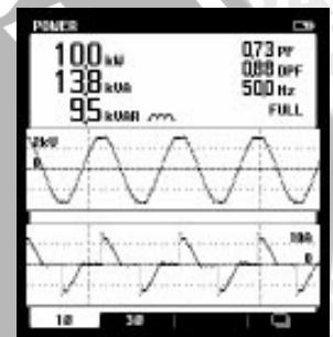
• Watts, power factor, displacement power factor (Cos \phi ), VA and VAR
