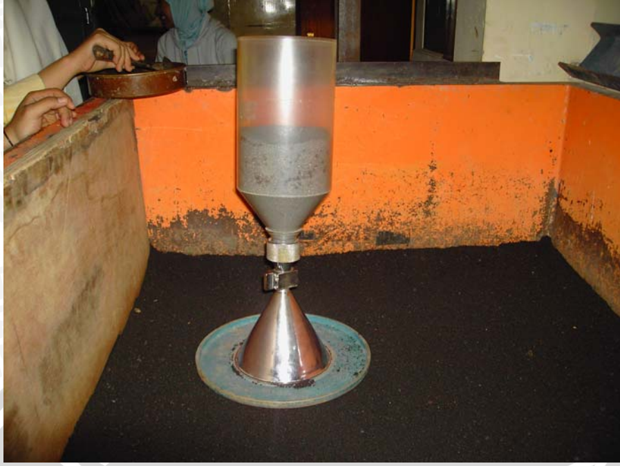
Uji kerucut pasir (sand cone test)
