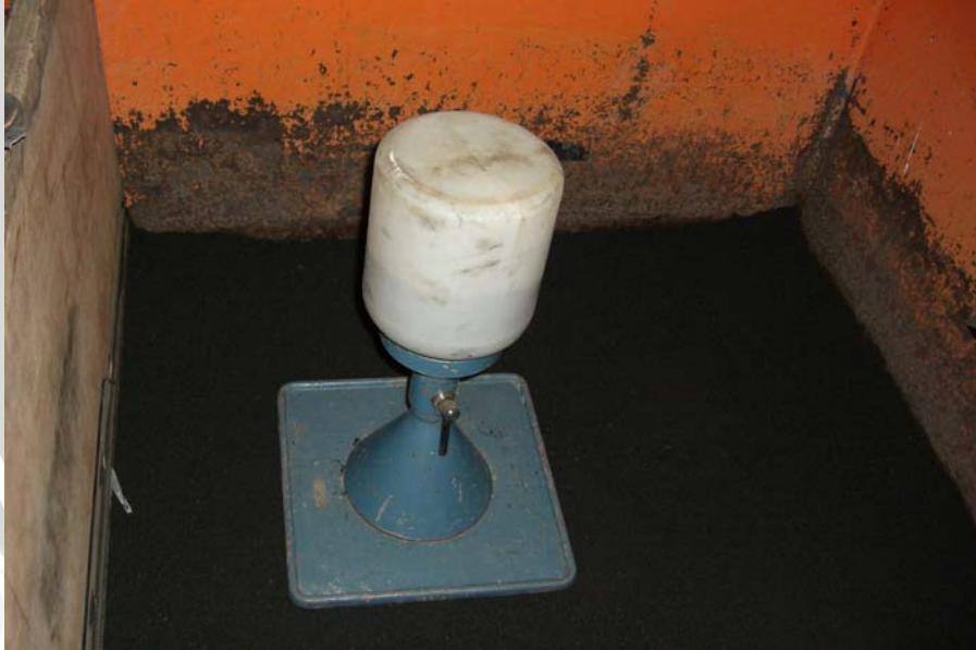
Uji kerucut pasir (sand cone test)
