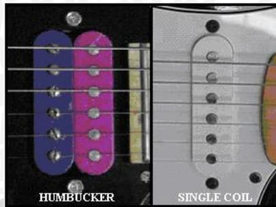
Gambar 2.5. Tipe Pickup Humbucker dan Single Coil
