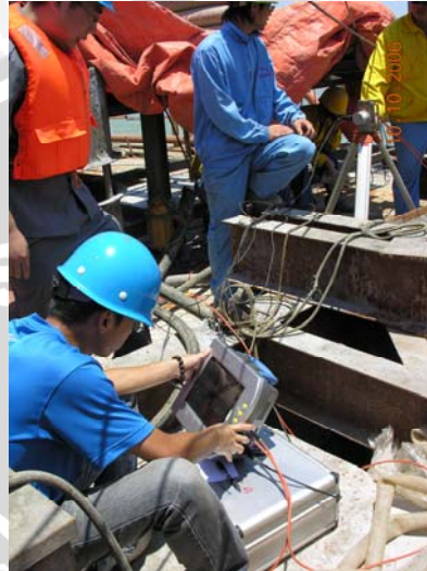
Gambar 2.13 Computer and automatic data acquisition system (Dokumentasi PT LAPI ITB)
