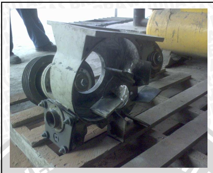
**Gambar 2.15.** *Rotary feeder.*
