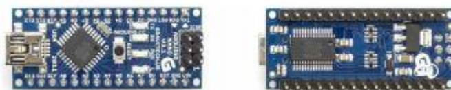
Gambar 2.4. Arduino Nano 3.0 (sumber : https://www.arduino.cc/en/Main/ArduinoBoardNano )
