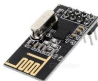
Gambar 2.5. Modul NRF24L01 (Sumber : http://www.robotshop.com/content/PDF/datasheet-wir020.pdf )
