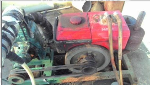
**Gambar 6.** Pompa Sumur Bor
