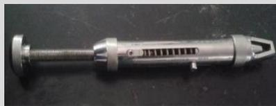
Gambar 4. *Hardness Tester*
