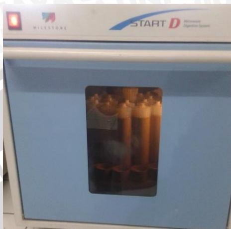
**Gambar 5.** *Microwave Digestion System*
