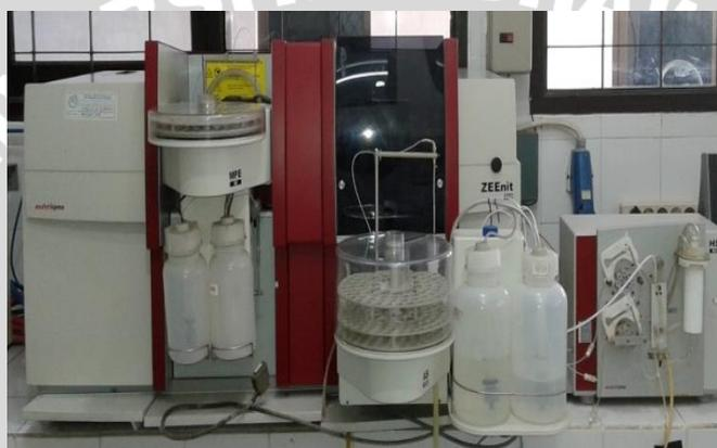
**Gambar 6.** AAS (*Atomic Absorption Spectrometry*)
