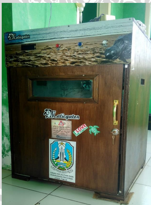
Gambar 3. Automatic turtle egg incubator (MATICGATOR)
