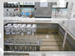
Inkubasi suhu 37 ^{\circ} C selama 5 menit
