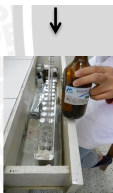
Penambahan 2 mL \text{Na}_2\text{CO}_3 75 g/L
