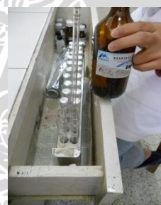
Penambahan 2 mL \text{Na}_2\text{CO}_3 75 g/L
