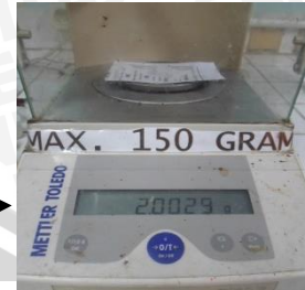
Penimbangan tablet kjeldahl sebanyak 2 gram
