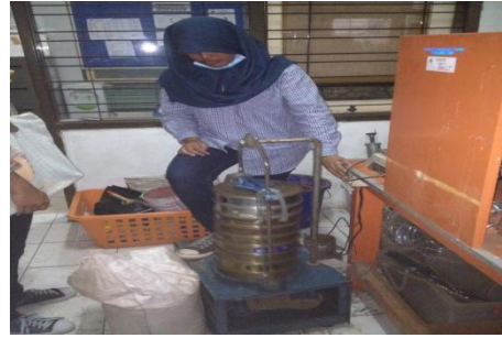
Analisis saringan ( sieve analysis )
