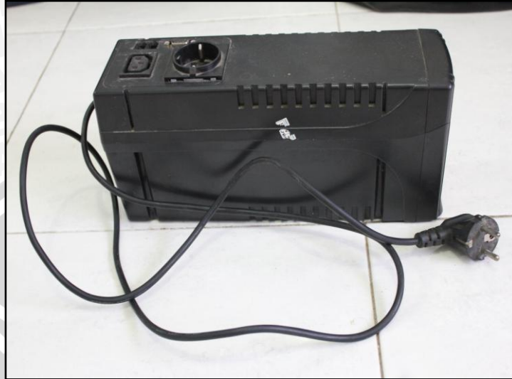
Gambar 12. Uninterruptible Power Supply (UPS)
