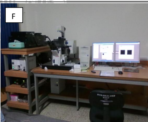
F: Perangkat Confocal Laser Scanning Microscope (CLSM) di laboratorium Molekuler dan seluler LSIH-UB.
