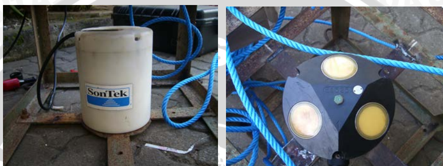
Gambar 9. ADCP Sontek Argonaut XR
