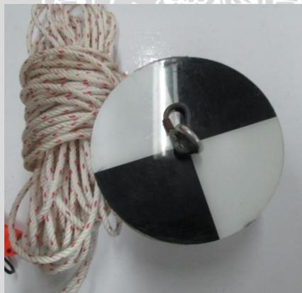
Gambar 8. *Secchi Disk*
