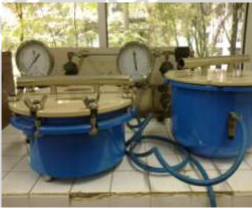
Gambar 11. Pengamatan pF 4,2 ( Pressure plate )
