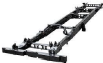
Gambar 2.3 Ladder frame Sumber : Sahu (2016)
