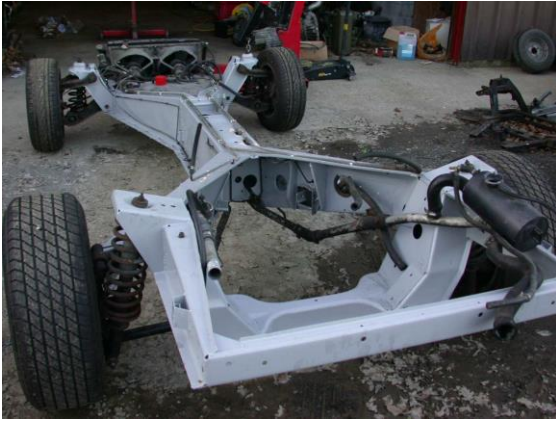
Gambar 2.6 Backbone chassis Sumber: Keith J. Wakeham (2009)
