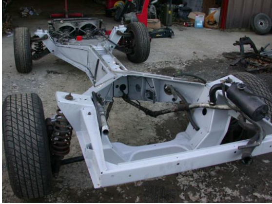
Gambar 2.6 Backbone chassis Sumber: Keith J. Wakeham (2009)
