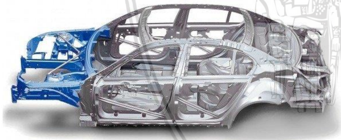
Gambar 2.4 Monocoque chassis Sumber : Sahu (2016)
