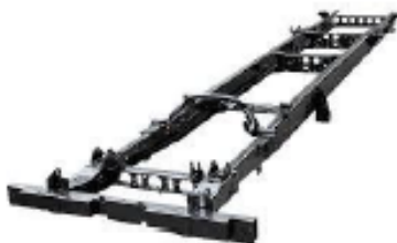
Gambar 2.3 Ladder frame Sumber : Sahu (2016)
