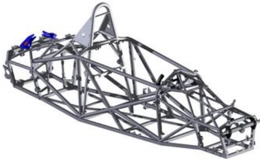
Gambar 2.5 Tubular Space Frame Sumber : Sahu (2016)
