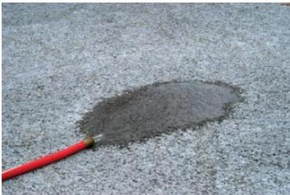
Gambar 2.1 Beton porous.
