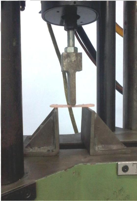
Gambar 7.6: Alat Universal Testing Machine Type PM 100 tarno
