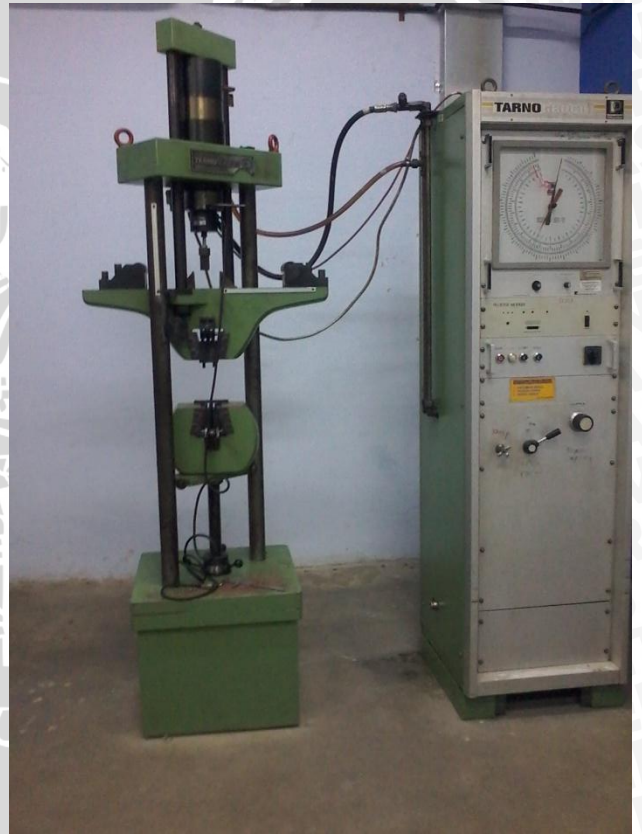
Gambar 7.6: Alat Universal Testing Machine Type PM 100 tarno
