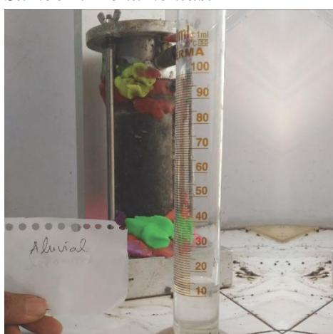
*Gambar 4.11 Permeabilitas sampel aluvial*
