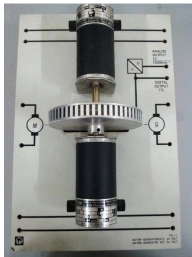
Gambar 3.15 Plant motor generator DC 73411
