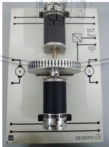
Gambar 3.15 Plant motor generator DC 73411
