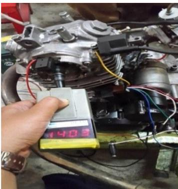
Gambar 3.4 *Tachometer mastech (HT-331)*
