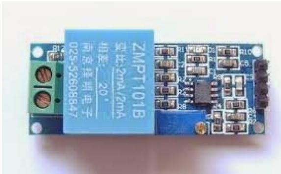
*Gambar 2.14* Sensor Tegangan ZMPT101B
