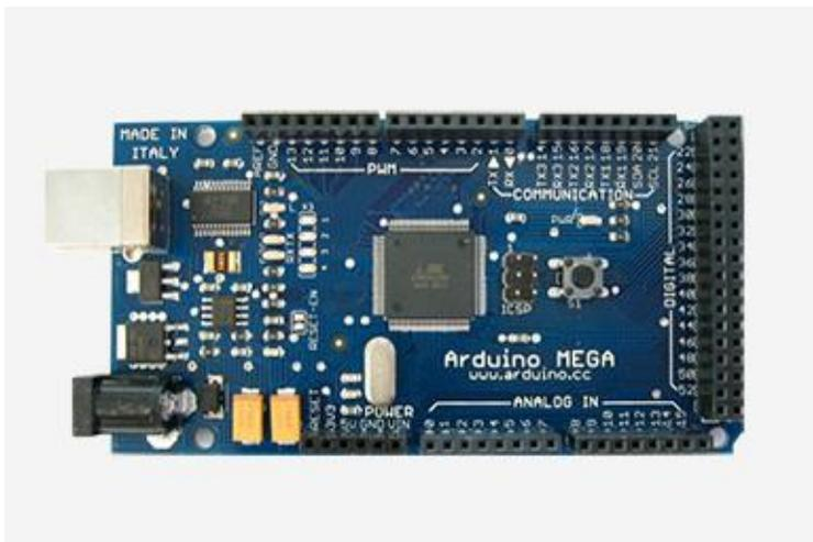
Gambar 2.13 Arduino Mega 2560
