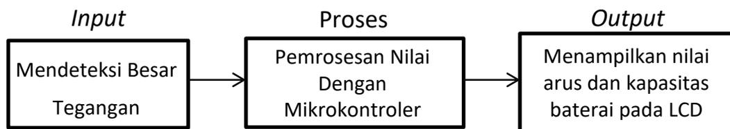
**Gambar 3. 2 Blok diagram sistem**
