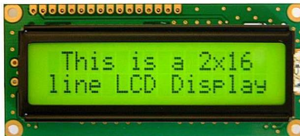
**Gambar 2. 3 LCD 16x2**
