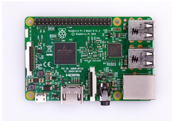
Gambar 2. 2 Raspberry Pi 3 [sumber : www.raspberrypi.org ]
